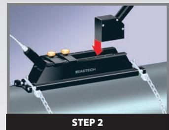
Since externally mounted sensors are the preferred design for transmitting signals through pipe or conduit, a new one piece **SpeedRail™** sensor mounting system was developed. Mounting of both sensors is quickly and accurately accomplished in two simple steps. Lock the self-aligning mounting rail to the pipe or conduit and load in the sensors.
